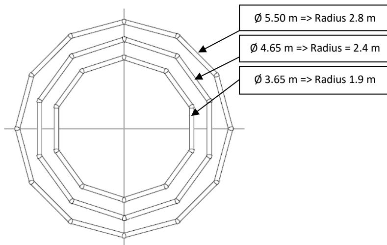
**The slab dimensions must exceed the pool dimensions by at least 30 cm all around the pool.**
