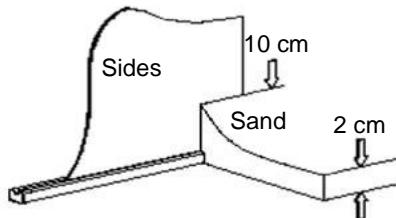
Cover the prepared ground with a geotextile film that goes 10 to 12 cm up the wall. Stick the film to the wall in various places using double-sided adhesive tape. The geotextile film prevents algae from spreading under the liner.
