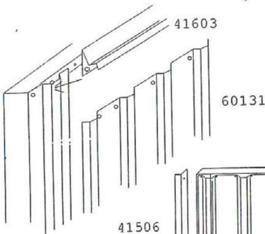
DOOR PELMET TO BE FITTED TO THE INSIDE OF 415.01, 415.05 AND 601.31 CLADDING PANEL
