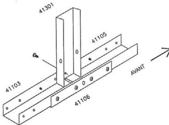
3. ASSEMBLER LE PROFILE AVANT DROIT 41203 ET LE PROFILE LATERAL DE COTE 41202 AU MONTANT STANDARD 41301 COMME INDIQUE CI-DESSOUS, A L'AIDE DE LA VISSERIE DE LA POCHETTE NO.1.
