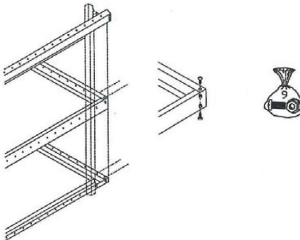
2. DE LA MEME MANIERE, FIXER LE PROFILE ARRIERE GAUCHE AU RAIL DE BASE ET AU PROFILE LATERAL.
