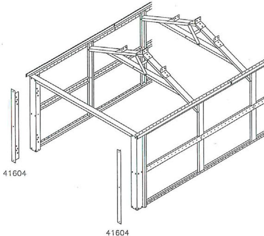
7. FIXER LES ANGLES DE LA STRUCTURE AVANT 41604 A LA STRUCTURE AVANT ET L'ATTACHEMENT DU PANNEAU D'ANGLE, AVEC DES VIS (SAC 1) ET DES RONDELLES EN FIBRE (SAC 7) COMME INDIQUE.
