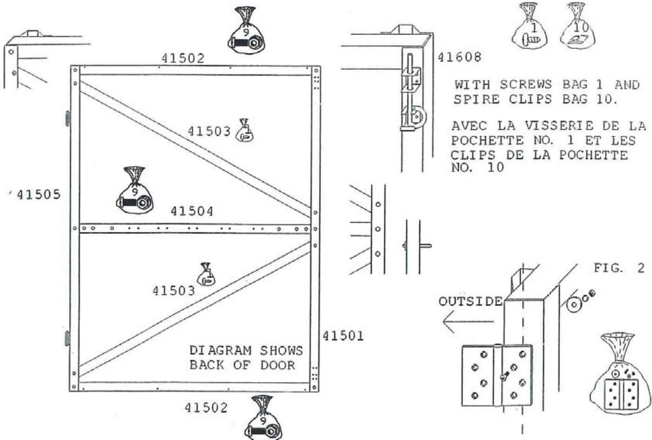
ATTENTION: ALWAYS ENSURE HOLES TO LOCATE HINGES ARE TOWARDS OUTSIDE OF DOOR ENSURE COMPLETED FRAME IS SQUARE.
