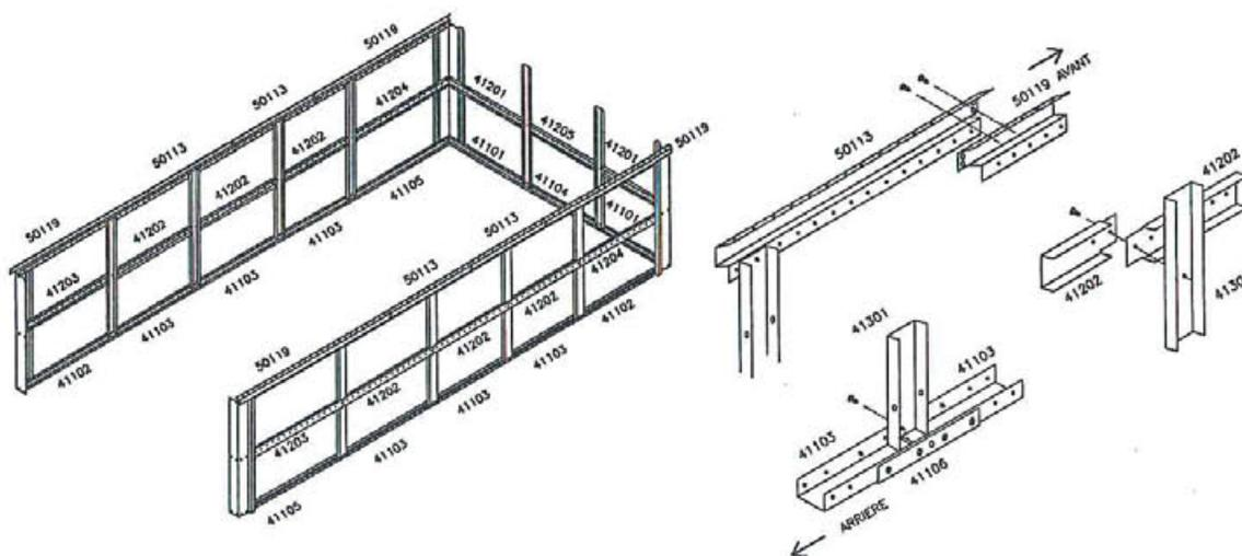
4. ASSEMBLER LES MONTANTS STANDARD 41301, LES DEUX PROFILS LATÉRAUX ENTAILÉS DE COTE 41202 AU TROU CENTRAL ET FIXER. ASSEMBLER DEUX PANNEAUX MURAUX 10118 AVEC VIS (SAC1) ET DES RONDELLES EN FIBRE (SAC 7).
